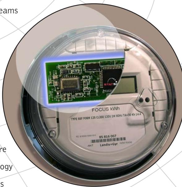
These devices (SensNODES™) report through a dynamic network manager (AiNODE™) to make up the StatSignal Pocket Network™ (LAN). The AiNODE serves as the transition point
